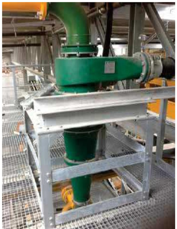
The heavy sand product is then pumped to a VV350-15-1 Stacker cyclone, the re-diluted underflow fed by gravity to a spiral bank of 8/8SC21/5/B/3 for heavy particle removal.
